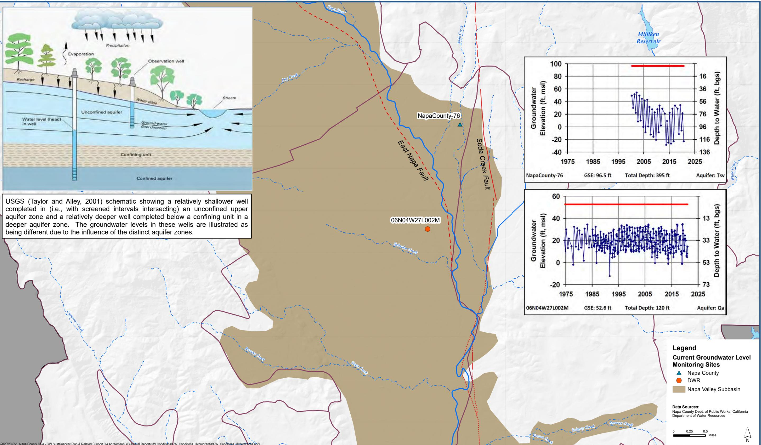
USGS (Taylor and Alley, 2001) schematic showing a relatively shallower well completed in (i.e., with screened intervals intersecting) an unconfined upper aquifer zone and a relatively deeper well completed below a confining unit in a deeper aquifer zone. The groundwater levels in these wells are illustrated as being different due to the influence of the distinct aquifer zones.
