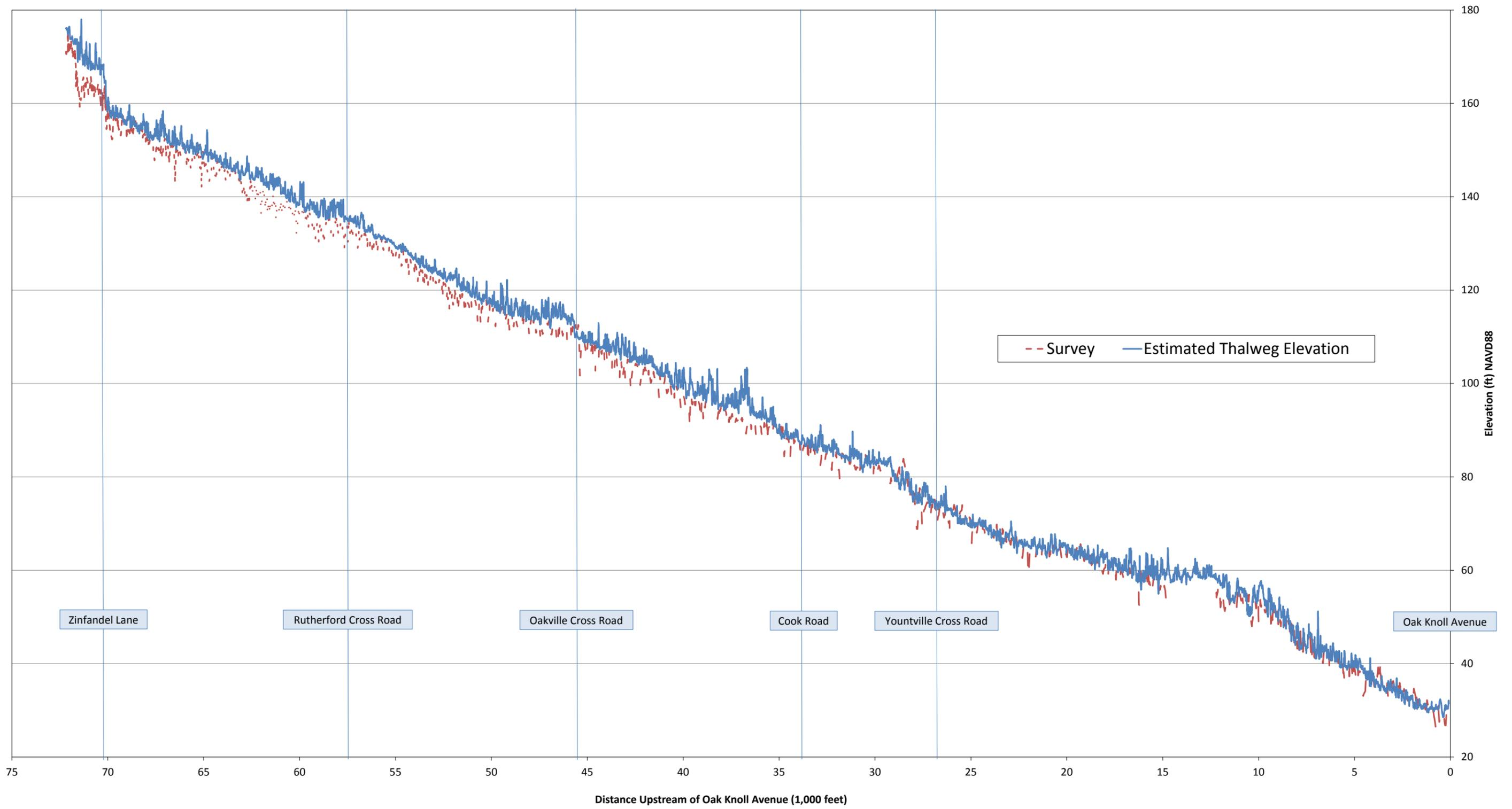
**Figure 7-4: Comparison of Estimated Stream Thalweg Elevation with Surveyed Data**
