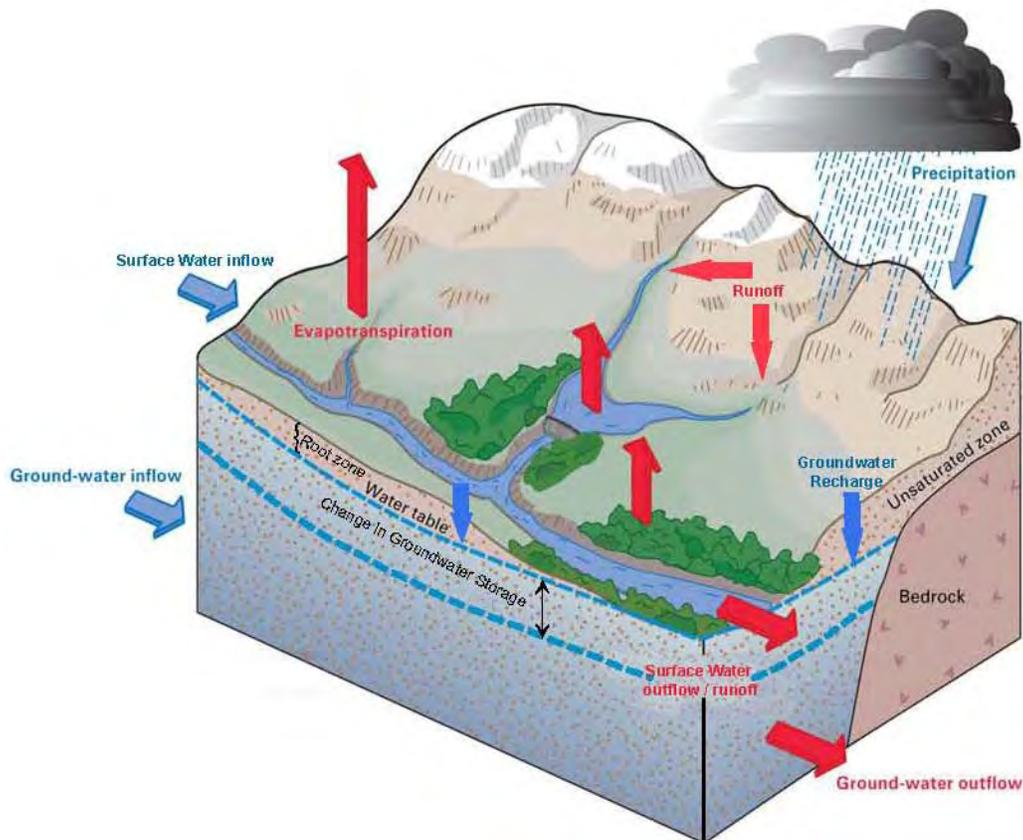
Figure 8-1. Conceptual Diagram of a Watershed Water Balance
